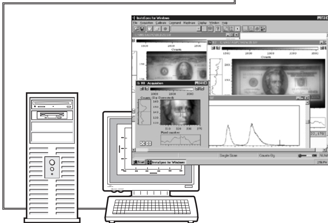
Fig. 7 UV source used to stimulate currency, yields a fluorescence spectrum. The long pass filter leaks the stimulation wavelength but attenuates sufficiently such that the dynamic range does not suffer. Data shown is overlaid fluorescent image and saved spectrum.
