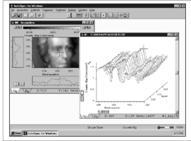
Fig.1 Image of fluorescing currency and relative intensity contour.
