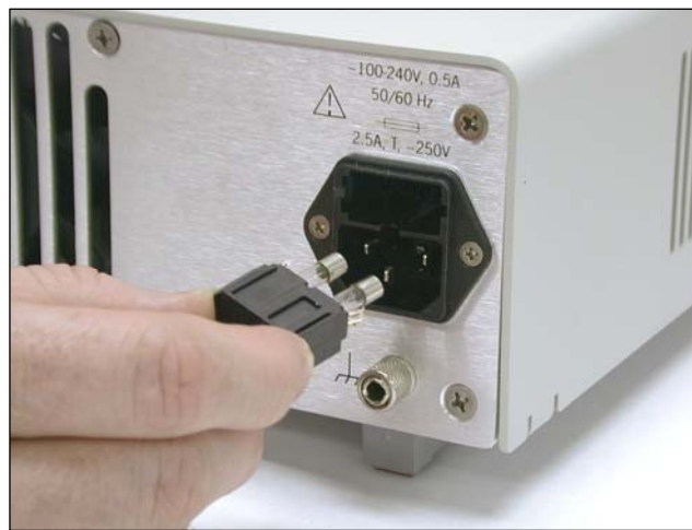
Figure 11. Removal of Fuse Block.
